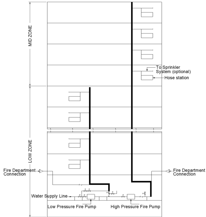
Figure 7.7/ Typical diagram for fire protection in different water supply zones of a tall building
